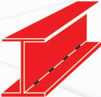
H-beam assembling (by auto Spot Welding)
